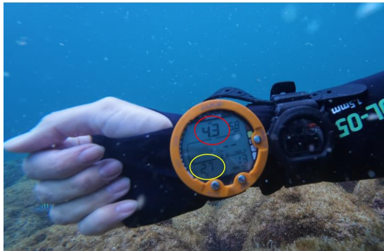
Figure 4: Diver displaying dive computer showing depth (red circle) and temperature (°C) (yellow). A digital watch may be used to monitor recording time (Photo: Talita Beneli).
